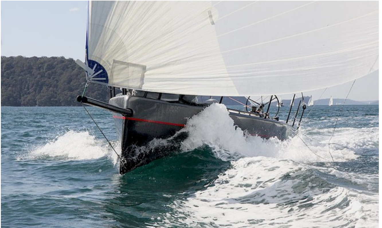
Purposeful and on a mission. Fuller bow helps to ensure she stays on her planing sections. - McConaghy MC38 - John Curnow
